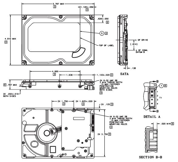
Figure 3. Mounting dimensions
